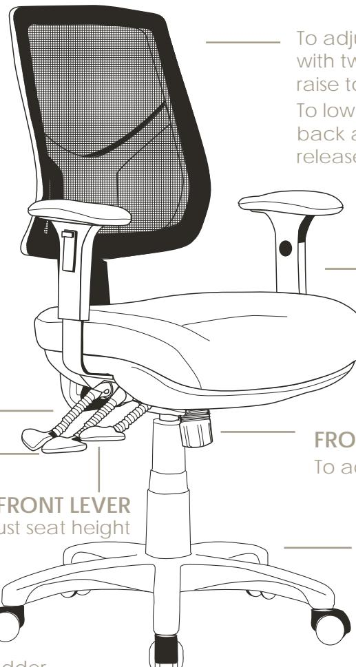
To adjust back height hold back with two hands while seated and raise to desired height
