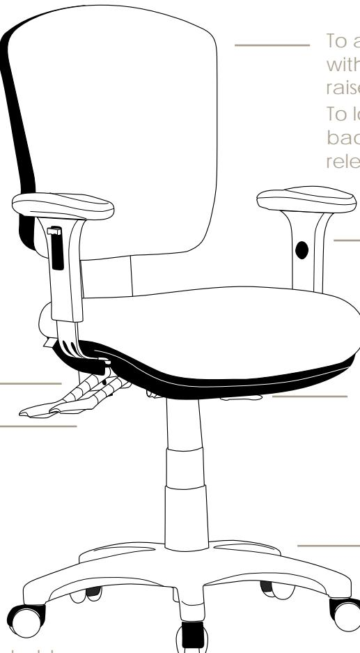
To adjust back height hold back with two hands while seated and raise to desired height
